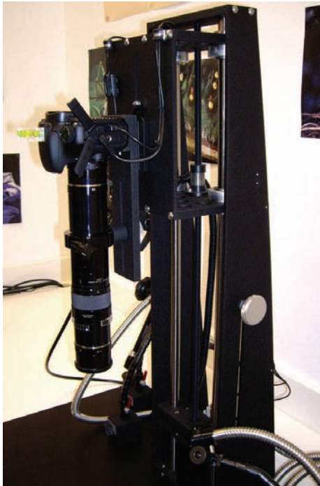
Left: Camera with in-line microscope on patented lift.
