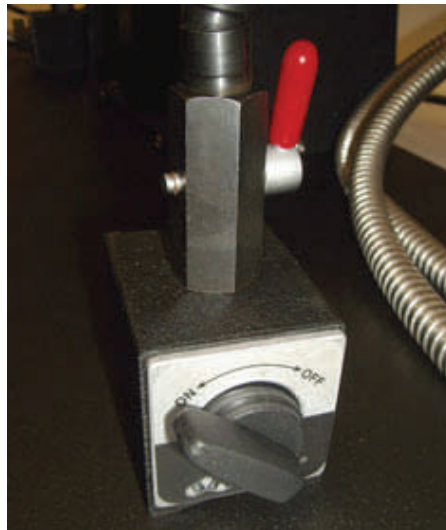
Above left: Fibre optic flash element with goose-neck support on magnetic base.
