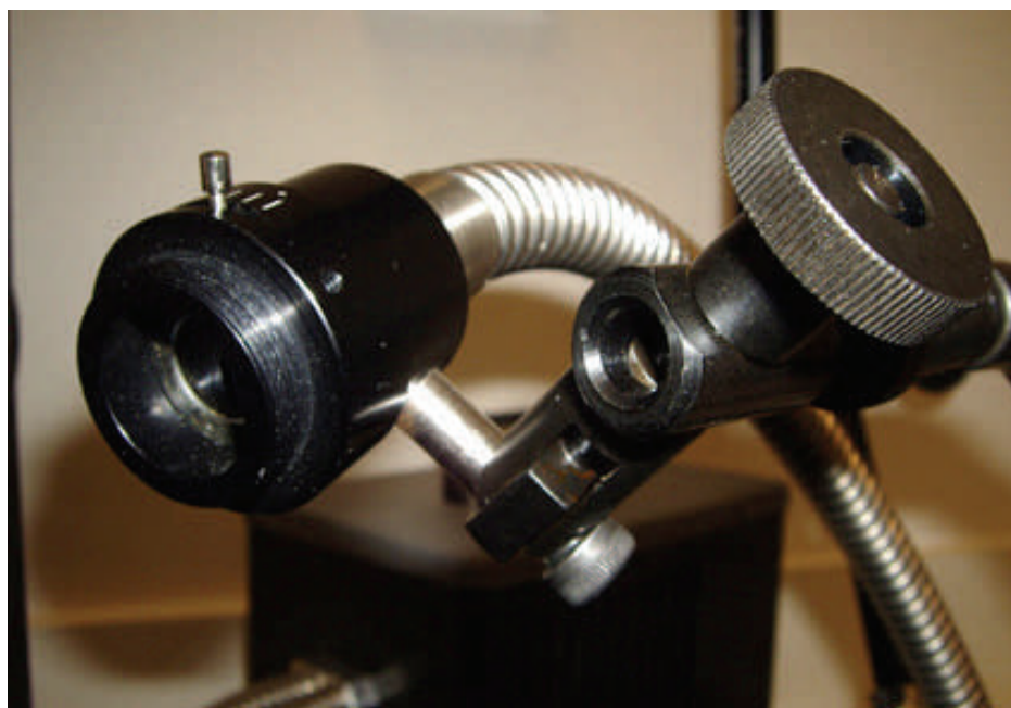
Below: Close-up of iris diaphragm at the end of the fibre-optic tube.
